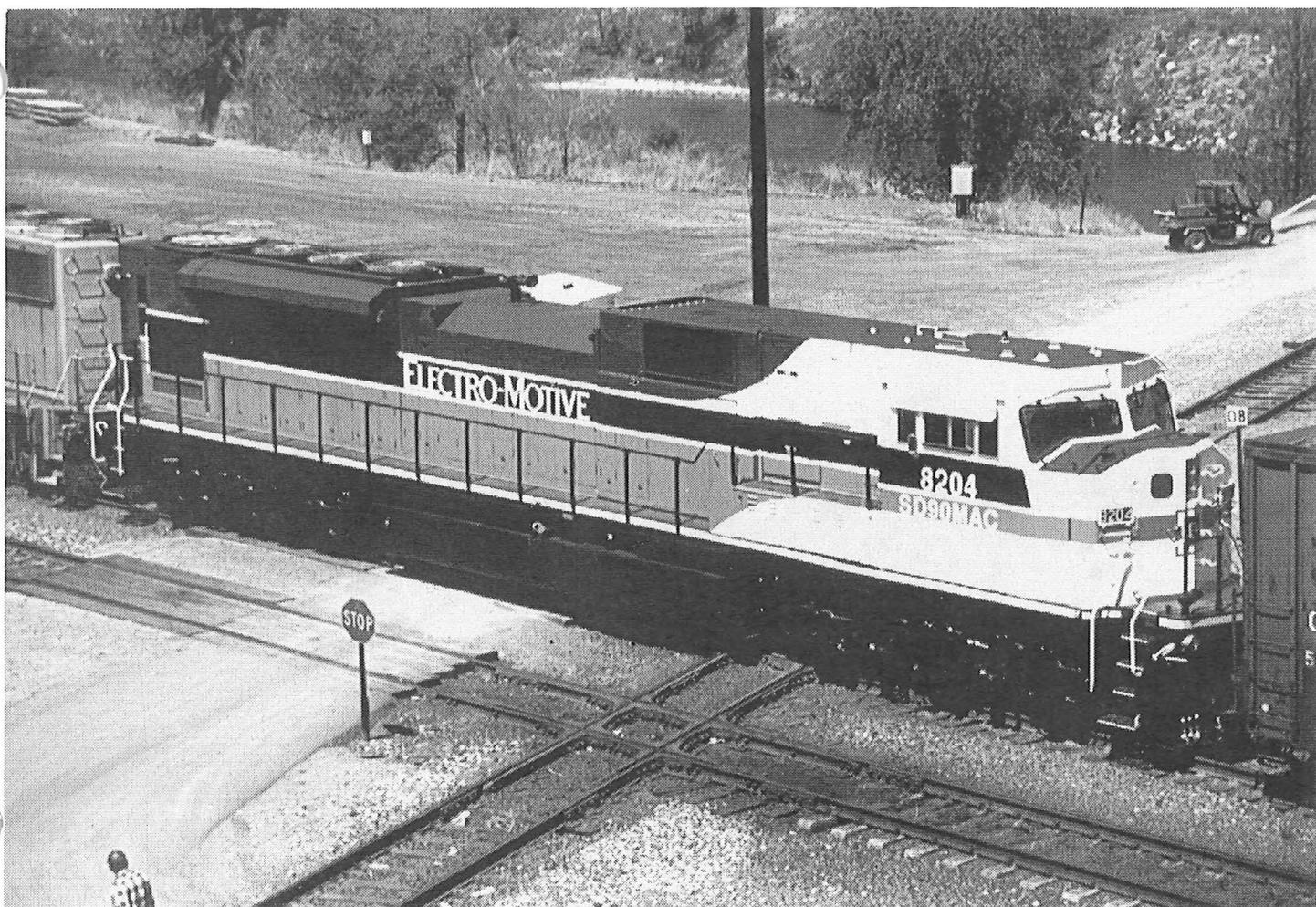
EMD SD90MAC #8204 was at the BNSF 23rd Street crossing on the BNSF train H-DENFTWI-09 enroute to the Transportation Test Center in Pueblo, CO, on May 9th, 1997. The unit sports EMD's 75th Anniversary paint scheme. This is EMD's newest 6,000 horsepower, AC-powered demonstration model. (Chip Sherman Photograph)
